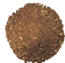
Clay topcoat plaster
